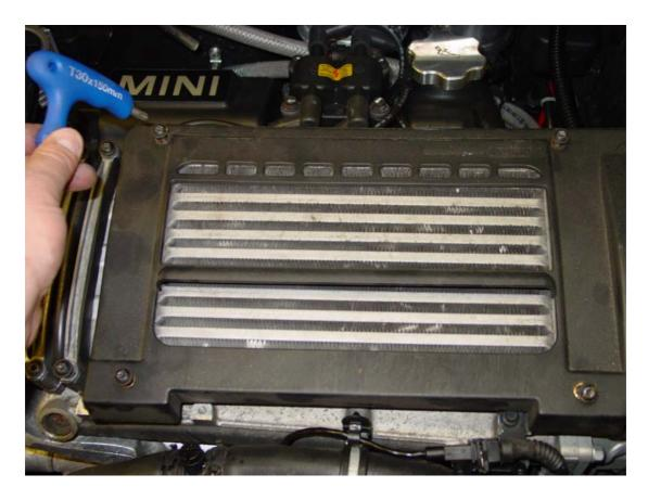
Now remove all of the steel support brackets from around the intercooler.
