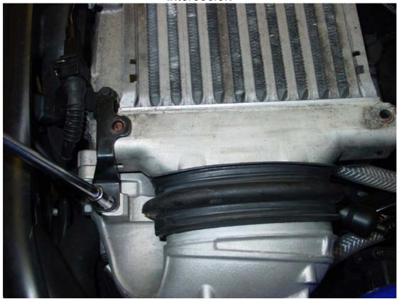
Remove three of the four clamps that secure the rubberconvoluted hoses, and then remove the Intercooler.
