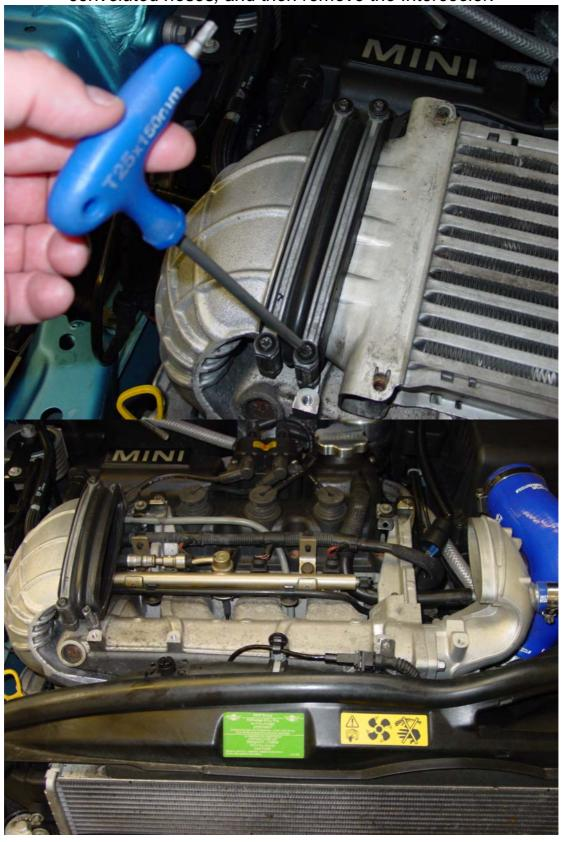
Remove the two steel brackets from the top of the Engine that used to secure the original intercooler.
